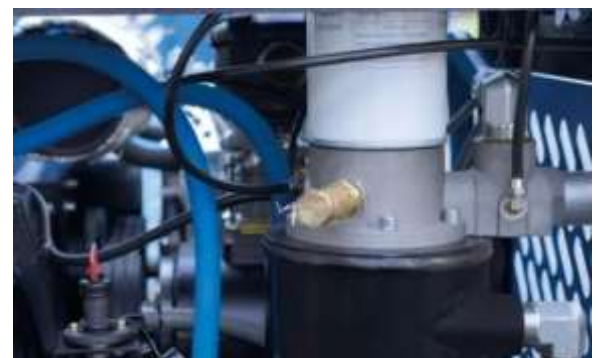
油分芯 Oil/air separator 外置油分芯，更换便捷
