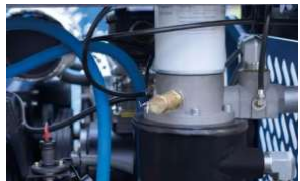
External oil separator External oil separator core, easy to replace
