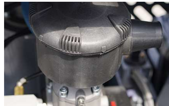
Air filter removing impurities and particulate matter
