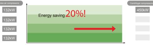
Generally, the larger volume, the higher efficiency. One centrifuge can save about 20% energy when replacing several small screws.
